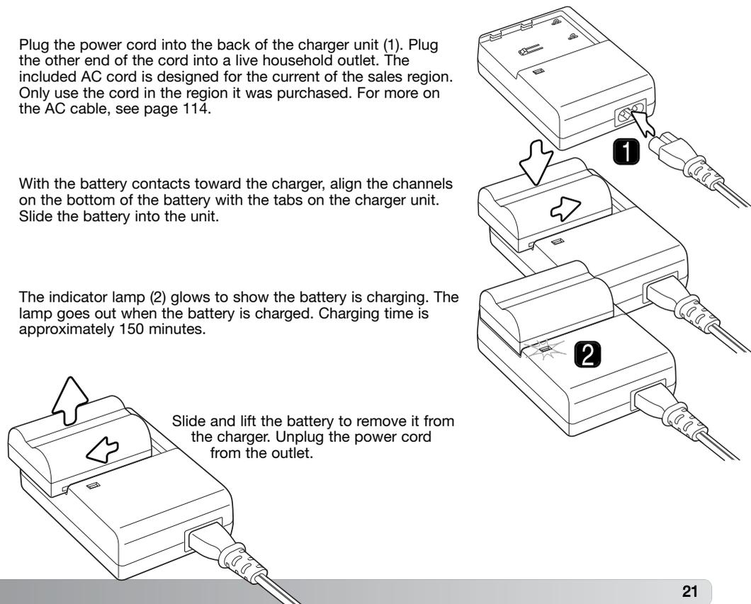
Slide and lift the battery to remove it from the charger. Unplug the power cord from the outlet.
