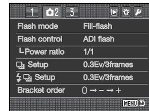
The camera automatically switches from ADI metering to pre-flash TTL when the autofocus system is prevented from focusing. When using the Macro Twin Flash 2400, Marco Ring flash 1200 or a wireless or off-camera flash unit, flash control is set to pre-flash TTL.
