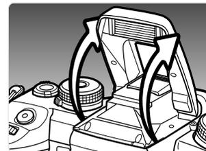
To use the flash, simply pull up the unit by the tabs on each side. The flash position must be set manually, and once up, the flash unit always fire regardless of the amount of ambient light. The flash mode is changed with the recording menu (p. 71).
