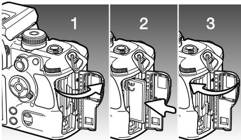
1. Open the card-slot door in the direction indicated.
