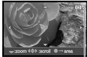
The controller's four-way keys scrolls the magnified area. The locator (2) indicates the portion of the image displayed. The rear control dial changes the magnification.
