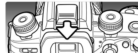
Slide the accessory-shoe cap off as shown. Mount the flash unit on the accessory shoe by sliding it forward until it stops.
