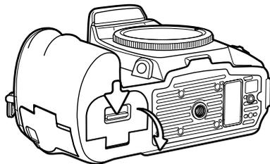
Insert the battery with the battery contacts first. Push the battery into the chamber until the battery latch clicks into place.
