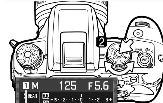
Camera settings are recalled with the exposure-mode dial.
