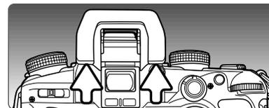
Carefully slide the eyepiece cup from around the viewfinder frame by pushing on each side of the cup.
