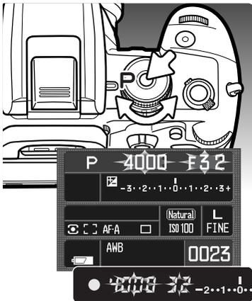
Program exposure is set with the exposure-mode dial (p. 39). Like full-auto program, program controls both the shutter speed and aperture required for each exposure. The operation is the same as described in the basic recording operation section on page 28. However, unlike full-auto program, functions set in this mode do not reset when the position of the exposure-mode dial is changed.
