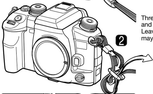
Thread the tip of the strap through the holder ring and the inside of the buckle and pull to tighten (2). Leave some slack in the camera strap so the tip may be threaded through the buckle easily.
