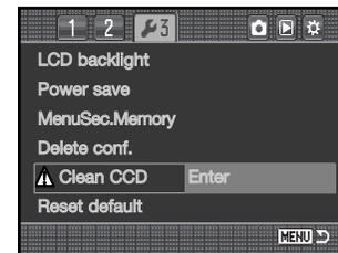
Before the CCD is exposed, a confirmation screen appears; choosing "Yes" executes opens the shutter and mirror, "No" cancels the cleaning operation.
