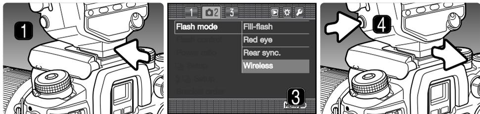
1. Remove the accessory shoe cap (p. 117) and slide a Program 5600HS(D) or 3600HS(D) flash on the accessory shoe until the safety lock engages.
