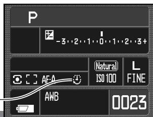
Confirm the memory card has enough storage capacity for the series by comparing the number of frames in the interval series with the number of recordable images displayed on the frame counter. Image size and quality settings can be changed to increase the number of pictures that can be saved on the memory card.
