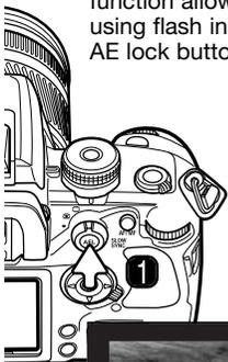
Frame the exposure target in the viewfinder depending on the metering mode in use (p. 50). Press and hold the AE lock button (1) to lock the exposure; the shutter speed and aperture are displayed and the AEL indicator is displayed in the viewfinder and on the monitor. Release the button to cancel the lock.
