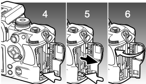
4. To eject a card, open the card-slot door, and press and release the card-eject lever to extend it.
