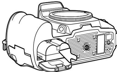
To remove a battery, slide the battery latch to the side of the battery chamber; the battery will spring out.
