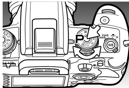
While pressing the Dial Lock Release, turn the exposure dial to the program (P) position. The camera controls the exposure system.
