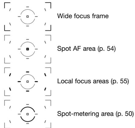
The spot AF area and local focus areas are illuminated briefly to indicate the point of focus when the focus is locked.
