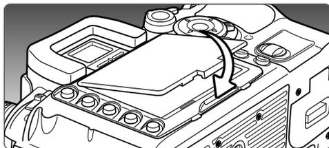
To remove the panel, lift from the bottom.
