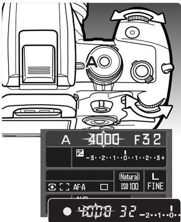
Aperture priority is set with the exposure-mode dial (p. 39). The photographer selects the aperture and the camera sets the appropriate shutter speed to ensure correct exposure.
