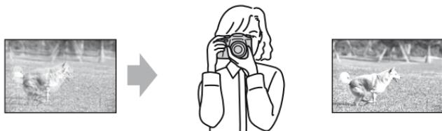
In a dark location, using the flash allows you to take a bright picture even of a subject in dim light and it also helps to prevent camera shake.
