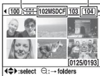
In each folder, six frames of image are displayed on the LCD monitor (File browser index). You can move frames around with **▲/▼/◀/▶** on the controller. This is useful when you want to scan the images to find the one you want.
