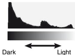
A histogram is the luminance distribution that shows how many pixels of a particular brightness exist in the picture. The histogram display of this camera shows the brightness on the horizontal axis (left side is black, right side is white) and the number of pixels on the vertical axis. The exposure compensation will change the histogram accordingly. Below is an example.
