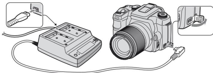
To connect the adaptor, set the POWER switch of the camera to OFF, flip open the cover, and insert the plug of the AC Adaptor/charger into the DC-IN terminal.
