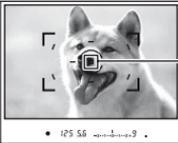
A photograph of a dog's face with a small square frame in the center. A label 'Spot focus frame' points to this frame. <ul style="list-style-type: none"><li>• When you look into the viewfinder, the spot focus frame is illuminated briefly.</li></ul>
