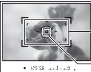
A photograph of a dog's face with a 3x3 grid of frames overlaid. One frame in the center is highlighted with a larger square, and a label 'Local focus frame' points to it. A label 'Spot focus frame' points to the center of the grid. <ul style="list-style-type: none"><li>• When you look into the viewfinder, the selected focus frame is illuminated briefly.</li><li>• After shooting, frame selection is still available. Be sure not to press the controller unless it is necessary.</li></ul> |
