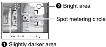
The indicator displays are as follows when the AEL (AE lock) button is pressed.
