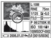
When the image has a high-key or low-key portion, that portion is illuminated on the histogram display (Luminance limit warning).
