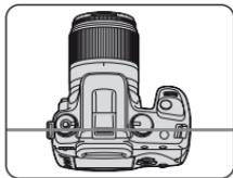
The horizontal line in the illustration shows the location of the CCD\* plane. When you measure the exact distance between the camera and the subject, refer to the position of the horizontal line.
