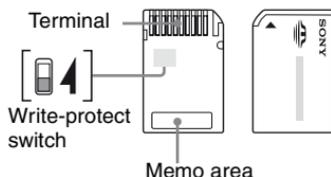
Some “Memory Stick Duo” cards do not have a write-protect switch. On “Memory Stick Duo” with this switch, the position and shape may vary depending on the “Memory Stick Duo”.
